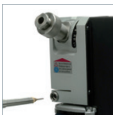
Precise adjustment of the electrode's stick-out.
