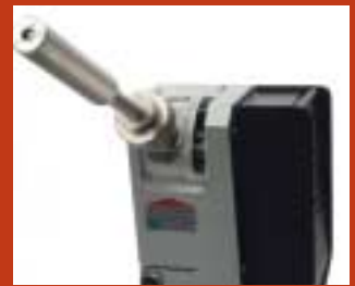
Adjustable grinding angle from 15-180° (included angle).
