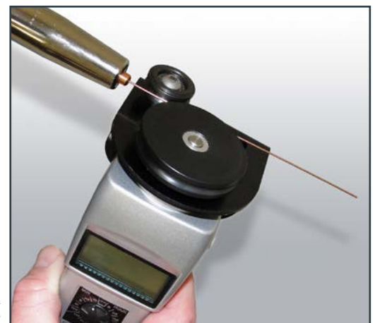
HHSS-12 obtaining measurement at the torch end
